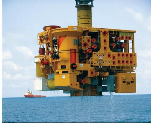
LEFT: FMC's subsea processing systems, like the pictured equipment installed at Statoil's Tordis field in the North Sea, perform separation of oil, gas and water on the seabed, helping customers increase production and recovery rates.
